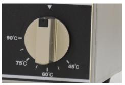
The temperature is controlled by an adjustable temperature dial which ranges from 45°-90°Celsius.
